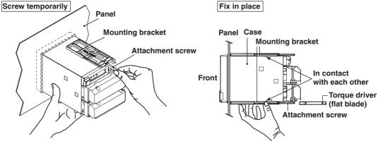
(The figure shows the case when the mounting brackets are used on the top and bottom of the case.)
